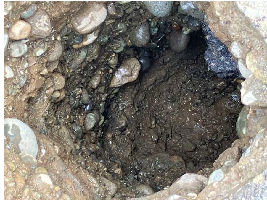
Photograph 4: Typical view of soils encountered from 0.3-1.8mbs.
