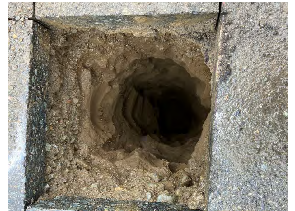
Photograph 6: View of TH23-01 with uniform sand from approximately 0.3 to 1.8m.
