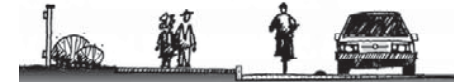
To accommodate cyclist, Bell McKinnon road should have a well maintained, 1 m wide shoulder on both sides of the road.
