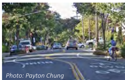
EXAMPLE: A bicycle boulevard incorporates traffic calming measures and provides clearly marked cycling routes.
